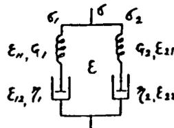
FIGURE 8 Two Maxwell elements in parallel connection.
