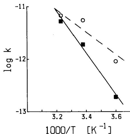
FIGURE 13 Arrhenius plot of the rate constant  $k$  of the bonding process for PSA-T and PSA-N. ○: PSA-N,  $\Delta H_{\text{bond}}^* = 10$  kcal/mole, ■: PSA-T,  $\Delta H_{\text{bond}}^* = 17$  kcal/mole.
