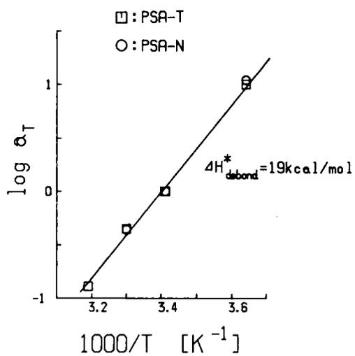
FIGURE 4 Arrhenius plot of the shift factor  $a_T$  for the lower velocity part of the curve of  $f$  vs.  $\log v$ .
