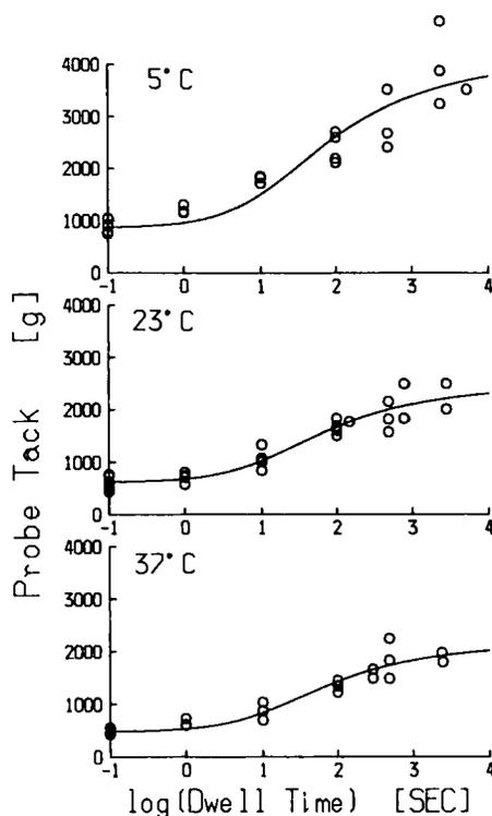
FIGURE 12 Probe tack *vs.* dwell time for PSA-N. Solid line is a curve of the 4th order rate equation.
