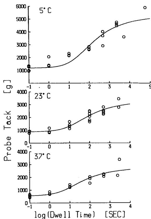
FIGURE 11 Probe tack vs. dwell time for PSA-T. Solid line is a curve of the 4th order rate equation.
