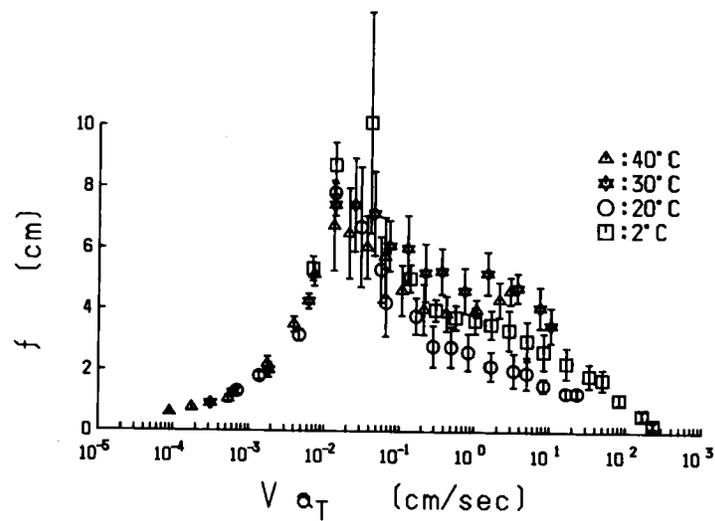
FIGURE 3 Master curve of  $f$  for PSA-T, reduced to 20°C.
